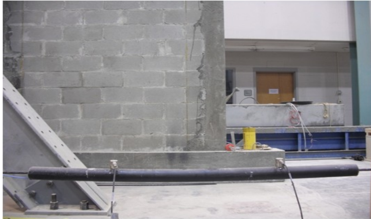
Figure 2. 8: Positioning of sensors on external PT specimens
